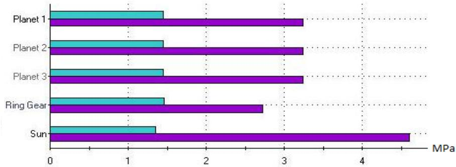
Figure 5: Gear contact safety factor and bending safety factor.
