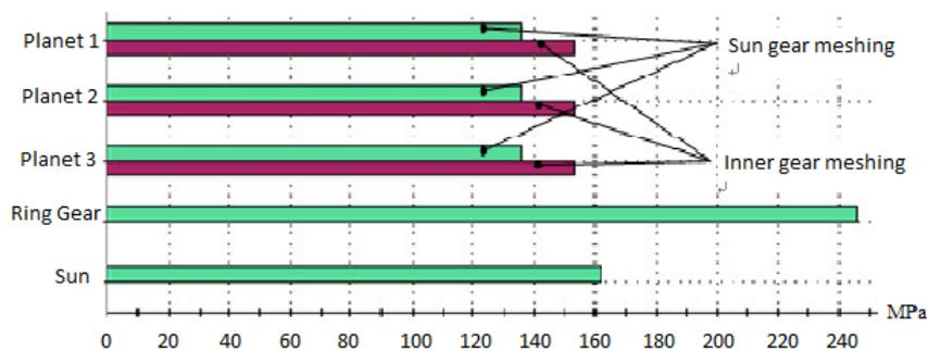
Figure 7: The maximum bending stress.
