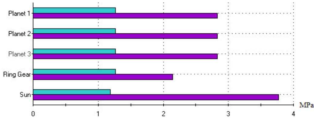
Figure 8: Gear contact safety factor and bending safety factor.
