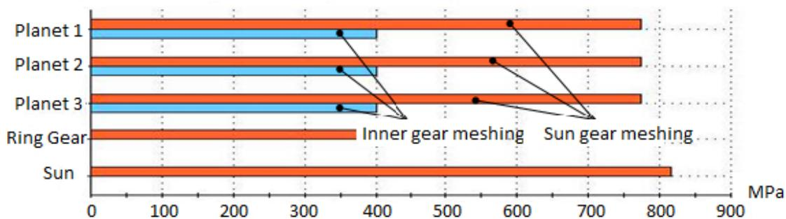
Figure 3: Maximum contact stress of gear.
