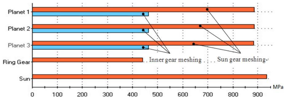
Figure 6: Maximum contact stress of gear.
